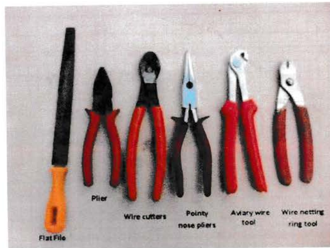
FIGURE 4: MAIN TOOLS FOR BUILDING CAGES
